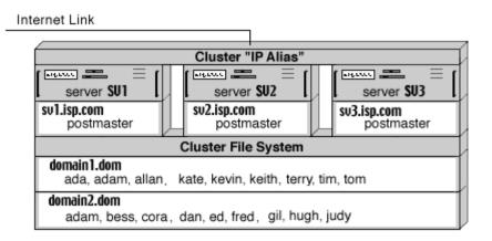
A Cluster OS can be used in a frontend/backend CommuniGate Pro Cluster configuration, too. In this case, one OS Cluster is used for CommuniGate Pro frontend Servers, utilizing the IP Aliasing load balancing, and the second OS Cluster is used for CommuniGate Pro backend Servers, where the Cluster File System is employed:
