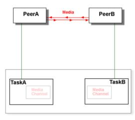
When the Tasks A and B are in the "bridged" state, one of the Tasks (Task A here) can receive Call Transfer (INVITE with Replaces) signal (delivered to it by the <u>Signal</u> module based on the Replaces field content):
