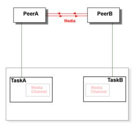
When the Tasks A and B are in the "bridged" state, one of the Tasks (Task A here) can receive a disconnect (BYE) signal from its peer, or it can quit for various reasons. In this case:
