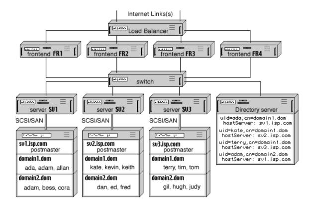
In a simplified configuration, you can connect Frontend Servers directly to the Internet, and balance the load using the DNS *round-robin* mechanism. In this case, it is highly recommended to install a firewall between Frontend and Backend Servers.
