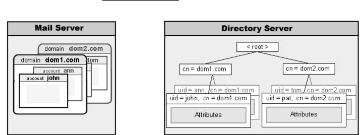
• The LDAP module received a ModifyRecord request from an LDAP client. The client asks the LDAP module to change attributes in theuid=john, cn=doml.dom record.
