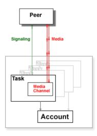
A Task can receive <u>Signals</u> from its peer, and it can send Signals itself. Signals can be used to end the current session, to update the session parameters, etc. Some of the Signals sent by the peer are processed by the Real-Time Application Environment itself, while other Signals are passed to the Task for processing.
