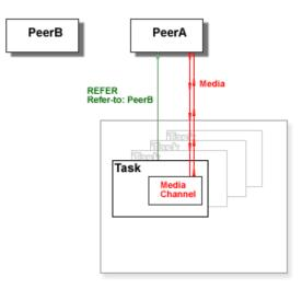
The INVITE signal initiated with the REFER signal can contain authentication information. The application program can instruct the Task:
