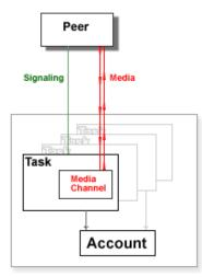
A Media Channel provides a *conversation space*. A Task can attach other peer media to the Task own Media Channel. This operation creates a conversation space (or a *conference*) that includes the Task own peer and all peers with media attached to this Task. Media sent by any peer in a *conversation space* is relayed to all other peers in that space, using the data mixing algorithms and parameters defined for that media type.
