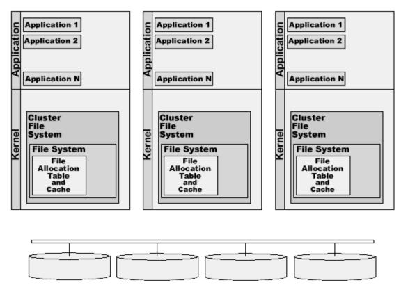
In this example, the Cluster File System is installed on several computers and serves requests from applications running on these computers.
