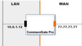
If your CommuniGate Pro Server is installed on a LAN behind a NAT/Firewall, the NAT/Firewall device should be configured to relay all connections on its communication (POP, SMTP, SIP, XMPP, etc.) ports to the CommuniGate Pro Server LAN address. Use this setting to specify the IP address your NAT/Firewall "relays" to CommuniGate Pro.
