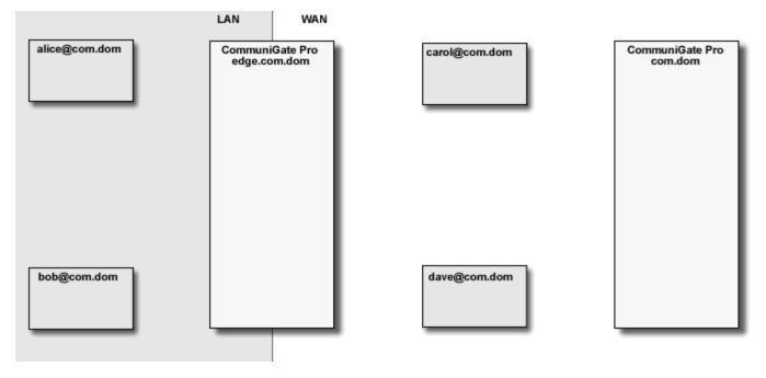
The CommuniGate Pro SIP Module detects "media loops", when a call placed from within LAN is proxied to WAN, and then proxied back to the same LAN. In this case the Media Proxies are removed, eliminating unnecessary overhead, and allowing SIP clients to communicate directly within one LAN, while proving registrar services outside that LAN.
