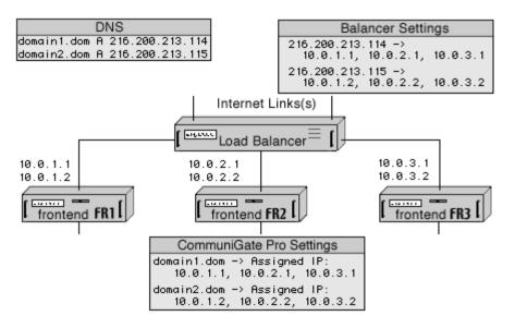
In this example, the Cluster is serving two Shared Domains: domain1.dom and domain2.dom, and the Cluster has three Frontend Servers. One IP Addresses assigned to each Shared Domain in the DNS server tables, and those addresses are external (Internet) addresses of your Load Balancer. You should instruct the Load Balancer to distribute connections received on each of its external IP addresses to three internal IP addresses - the addresses assigned to your
