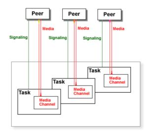
A Task with attached peer media can use its Media Channel to send media to its own peer and to all attached peers at once.
