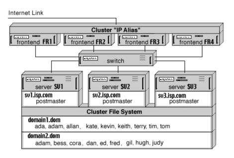
The Configuration of the CommuniGate Pro Dynamic Cluster does not depend on the type of the load balancing used (separate Load Balancers or IP Aliases), or on the type of the shared file system used (Network File System or Cluster File System).
