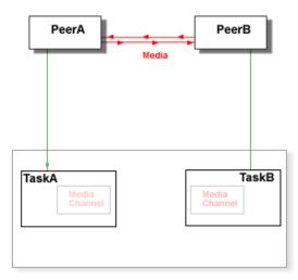
When the Tasks A and B are in the "bridged" state, one of the Tasks (Task A here) can receive a Call Transfer (REFER) signal
