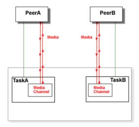
When the Tasks A and B are in the "bridged" state, one of the Tasks (Task B here) can receive a re-INVITE signal from its peer. The new media description in this signal request may ask the Task to change its media parameters (hold/resume, switching to a different media source, etc.). This re-INVITE signal is processed automatically, without any involvement of the application programs the Tasks are running:
