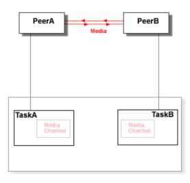
The Real-Time Application engine may choose to implement a Media Bridge using one Task Media Channel as a "media relay".
