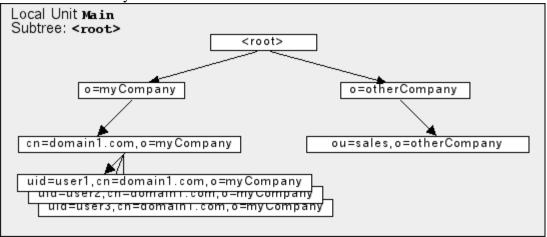
The diagram below shows the same directory stored in 2 Storage Units, with the entire o=MyCompany subtree stored in a separate Storage Unit LDAP1:
